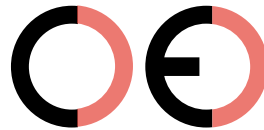
False CE Mark (too far)
